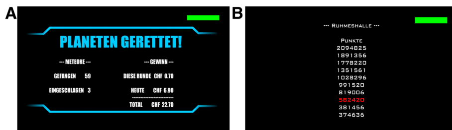
Fig. 4 ArmeoSenso-Reward feedback screens. a "PLANETEN GERETTET": planet saved. This screen is presented after each completed round. The number of meteors caught ("GEFANGEN", top) and meteors hitting the planet ("EINGESCHLAGEN", bottom) is indicated on the left. The monetary reward ("GEWINN") for the current round ("DIESE RUNDE", top), the current day ("HEUTE", middle) and the total amount of money gathered over the course of the study ("TOTAL", bottom) are displayed on the right. Note that a maximum of 1 Swiss Franc (CHF) can be won per round. b Hall of fame ("RUHMESHALLE") with the patient's top 10 scores. If the current score is in the top 10, it is highlighted in red
